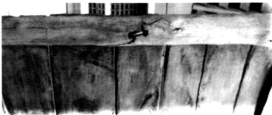
Figure 9. Detail showing the damage to the wood on a side part of Cheops boat
